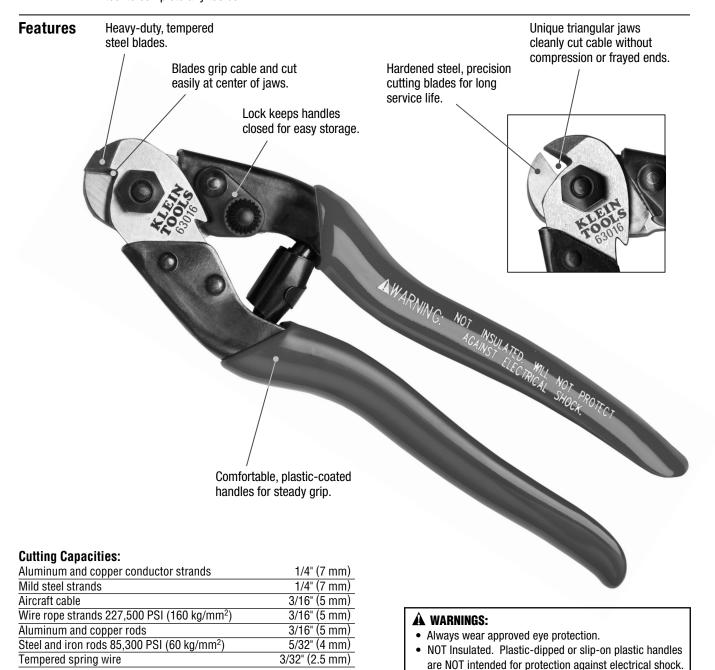
**NOTE:** Cut hard material only in the cutting triangle of the blades.
