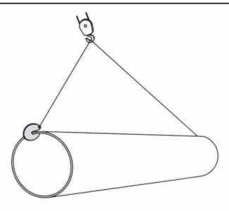
NOTE: Load must be able to support it's own weight under compression.
