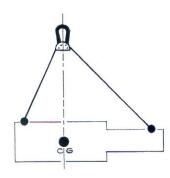
For loads that are heavier on one end, with the center of gravity off-center.
